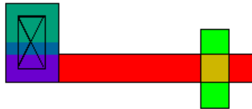
Contact rotated, fixed-angle wire
